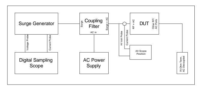
Figure 4, Combined RF and AC Port
